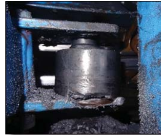
Roller severely damaged requiring replacement
